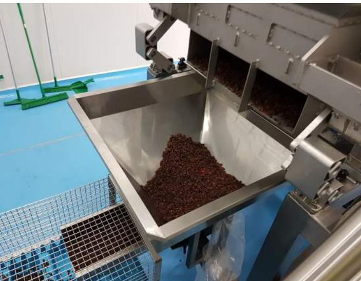
The Industrial Power Sieve is a vibratory hopper system that is used to break up and screen product. At ADM we developed the Industrial Power Sieve to break up clumped sultanas and raisins to improve the packaging process and product display quality.
