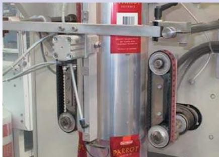
Lagged and glued belts have visible joins, an uneven finish, a weak bond and uneven wear. However the **Truly Endless** belts are moulded to create a stronger bond and accurate film feed. Superior in quality, with a ground finish, these specialty belts deliver an even wear for high performance applications.
